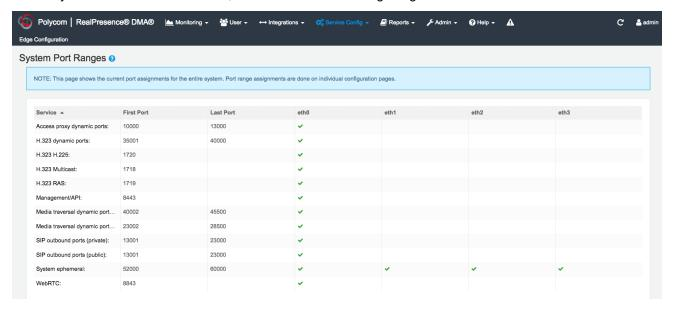
After installation, if you run the DMA Edge Wizard and specify the **Maximum number of simultaneous calls** as *x*, the default port ranges for each service will adjust to the total number of ports required to support *x* simultaneous calls. The system calculates the total number of ports required using the formula described in the <u>preceding table</u>. The following image shows the port ranges for 1000 simultaneous calls, with services bound only to eth0:
