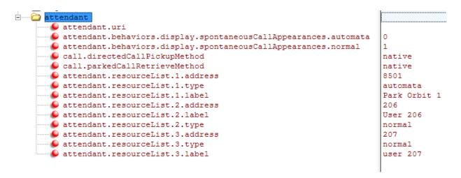
The above figure shows a configuration for 3 monitored resources using the static configuration method of BLF. One resource is using the Automata type which designates a behavioural change for that BLF vs the others commonly associated when monitoring IVRs or park orbits.
