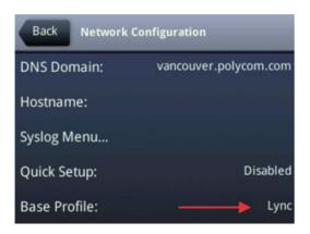
3 Select **Back > Save Configuration**. The phone automatically restarts and displays the Sign In screen. You can now Sign In or Out of Lync.
