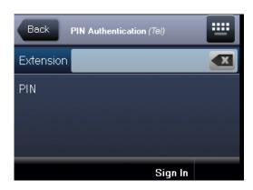
2 Enter the phone's extension and your PIN, and press **Sign In**. Press the **Exit** soft key to sign out and return to the idle screen.
